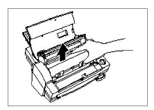
(3) Remove the film cartridge carefully.
